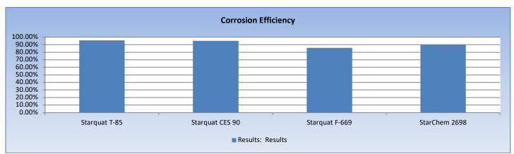
Testing performed on mild steel in HCl solution. Products were tested at 2 ppm. Corrosion efficiency calculated:
